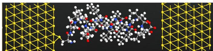
Electron transport calculations were performed on fragments using Atomistix Toolkit software (DFT/ double- $\zeta$  basis set)
