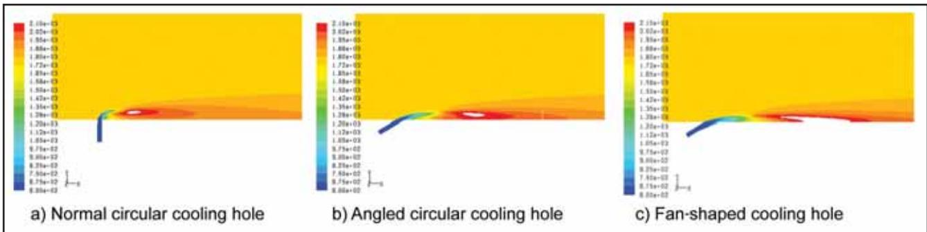
Figure 3a-c. Temperature contours on the midplane for  $\Phi = 1.5$ ,  $M = 1.0$ , air injection
