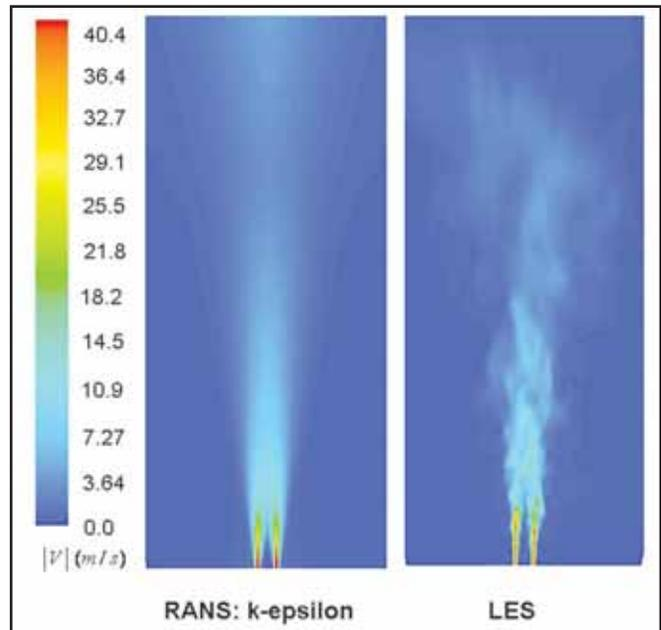
Figure 5. Contours of velocity magnitude at the  $y/d = 0$  plane, comparing  $k - \varepsilon$  and transient LES
