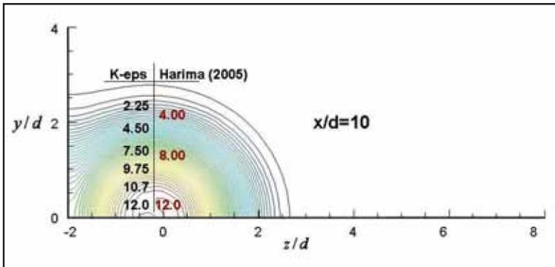
Figure 7. Turbulence intensity contour comparisons at  $x/d = 10$
