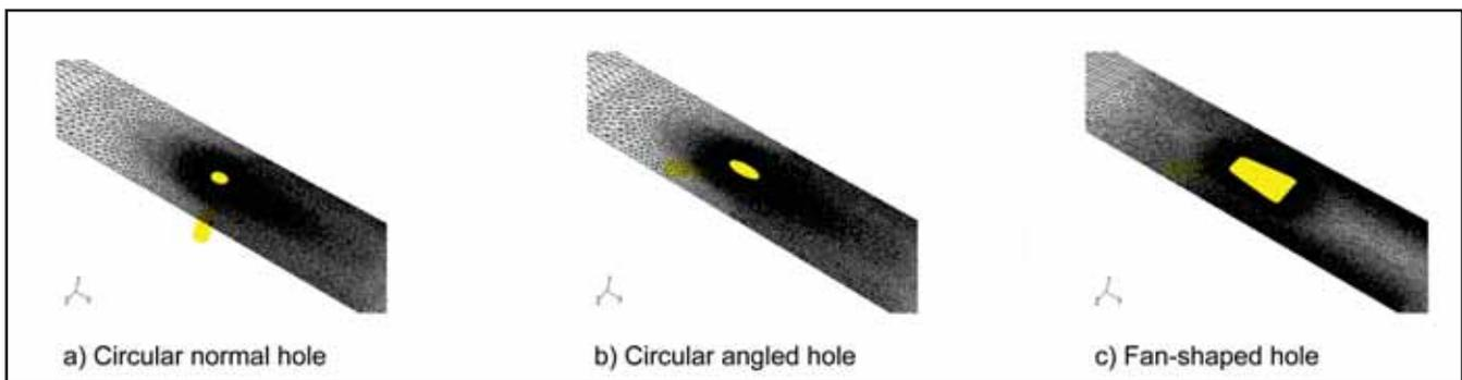
Figure 1. a-c Schematic of circular normal, angled circular, and fan-shaped hole meshes
