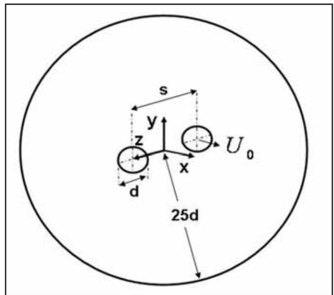
Figure 2. Lower base geometry ( $x/d = 0$ ) and inlet circular jet configuration including location of reference coordinate system
