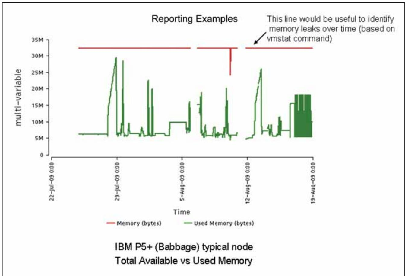
Figure 3. This report example shows Navy’s HPC system Babbage’s memory information. This metric identifies memory leaks over time
