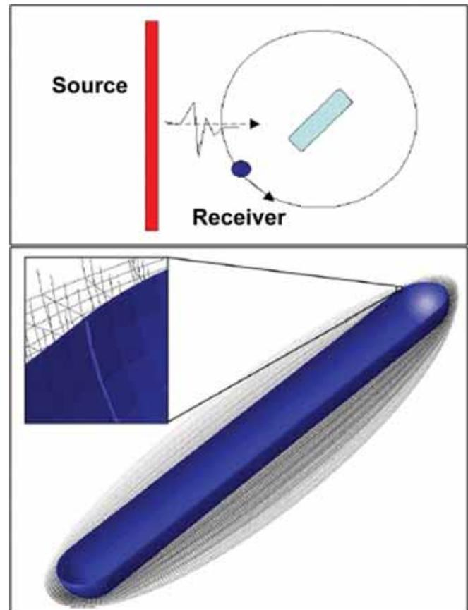
Figure 1. Scattering from an E50 shell: (a) schematic description of the problem and (b) view of 3-D finite element mesh “h1.” The refined “h2” mesh is obtained by splitting mesh edges by half
