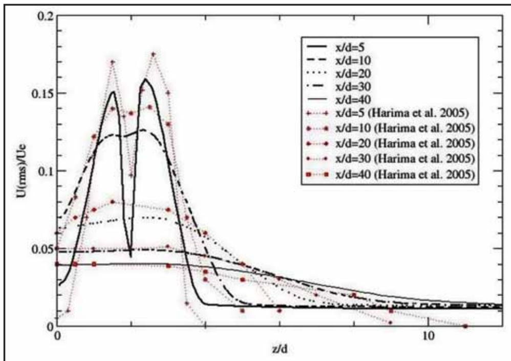
Figure 10. Streamwise variation of longitudinal turbulence intensity along the  $z$ -axis for  $S/d = 4$
