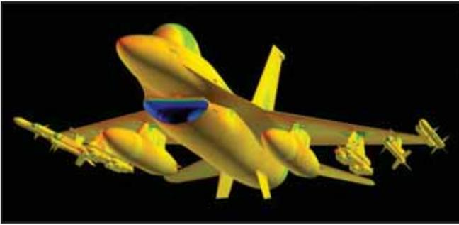
Figure 3. F-16 SDB flight-test configuration
