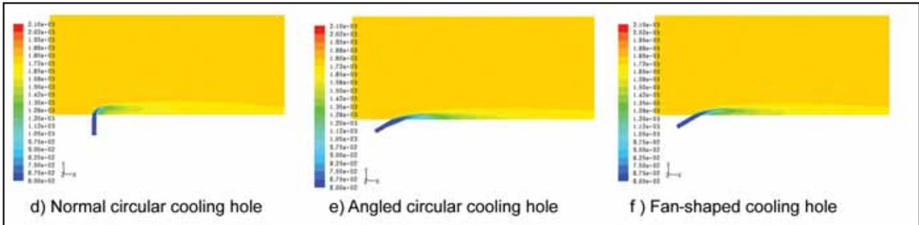
Figure 3d-f. Temperature contours on the midplane for  $\Phi = 1.5$ ,  $M = 1.0$ ,  $N_2$  injection
