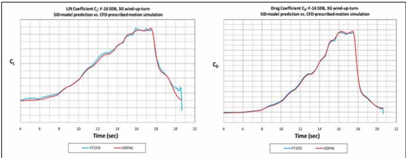
Figure 6.  $C_L$  and  $C_D$  results for a prescribed-motion 3G wind-up-turn in CFD and the corresponding SID-model prediction generated from a 10-second multi-axis computational training maneuver in CFD. Full-scale, static, time-accurate analysis of the F-22 in the clean aircraft configuration is also underway. Shown in Figure 7 is a static, time-accurate simulation depicting isosurfaces of vorticity colored by pressure at Mach 0.9
