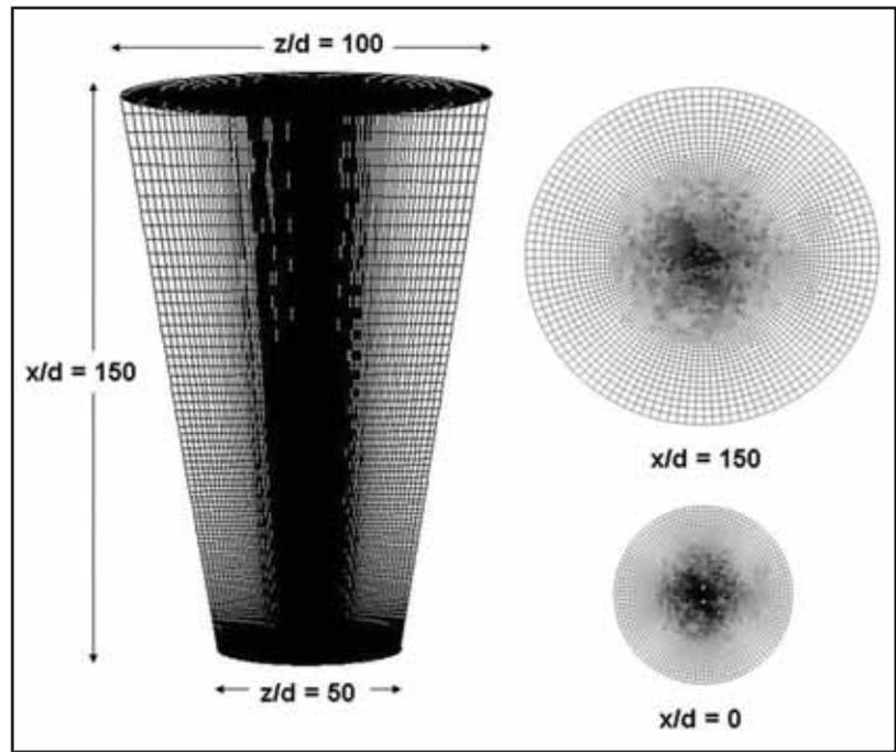
Figure 3. Representative hexagonal mesh ( $1.517E6$  elements) corresponding to jet spacing,  $S/d = 4$
