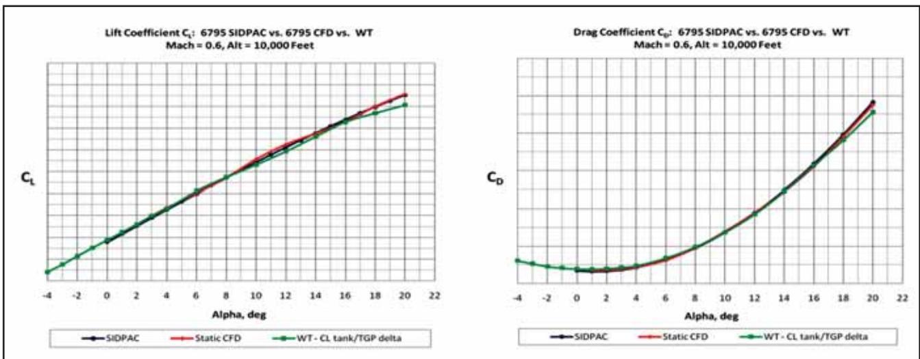
Figure 5.  $C_L$  and  $C_D$  results for the F16C SDB flight-test configuration. Plots are of a SID-model prediction, CFD-static results, and wind-tunnel results
