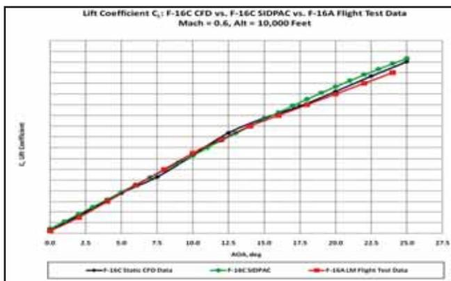
Figure 1. Comparative plots of lift coefficient for the F-16 using flight-test data and CFD simulations
