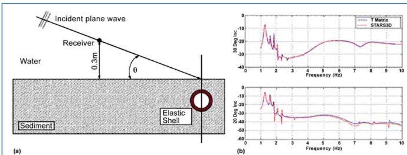
Figure 3. Scattering from an elastic spherical shell in sediment: (a) schematic description of the problem, and (b) comparison between STARS3D computations against the T-matrix method. The monostatic response is shown for 30 and 20 degree incident
