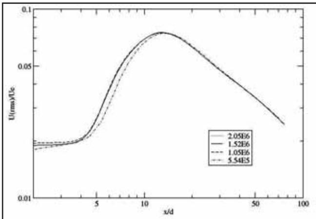
Figure 4. Sensitivity of the numerical solution to grid resolution
