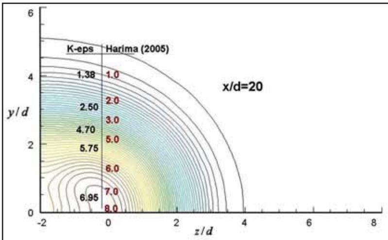
Figure 8. Turbulence intensity contour comparisons at  $x/d = 20$
