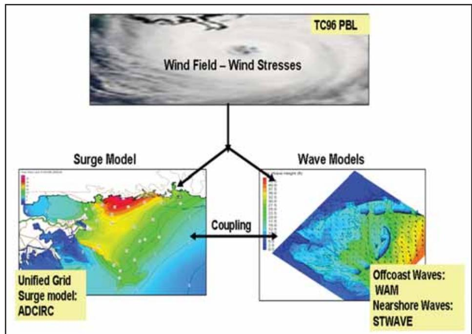
Figure 1. Diagram of modeling system for coastal inundation application
