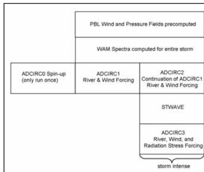
Figure 3. Coupled modeling system flow chart
