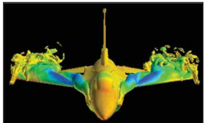
Figure 2. Image from a computational training maneuver for use with SID. Conditions are Mach 0.6, 10,000 ft, and 0 to 25 deg AOA
