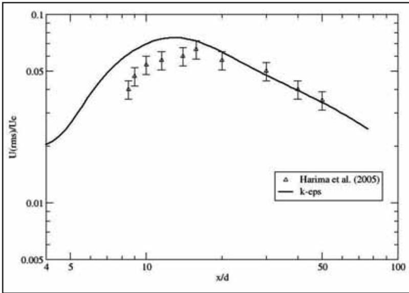
Figure 6. Experimental and numerical comparisons ( $k - \epsilon$ ) for the streamwise variation of turbulence intensity
