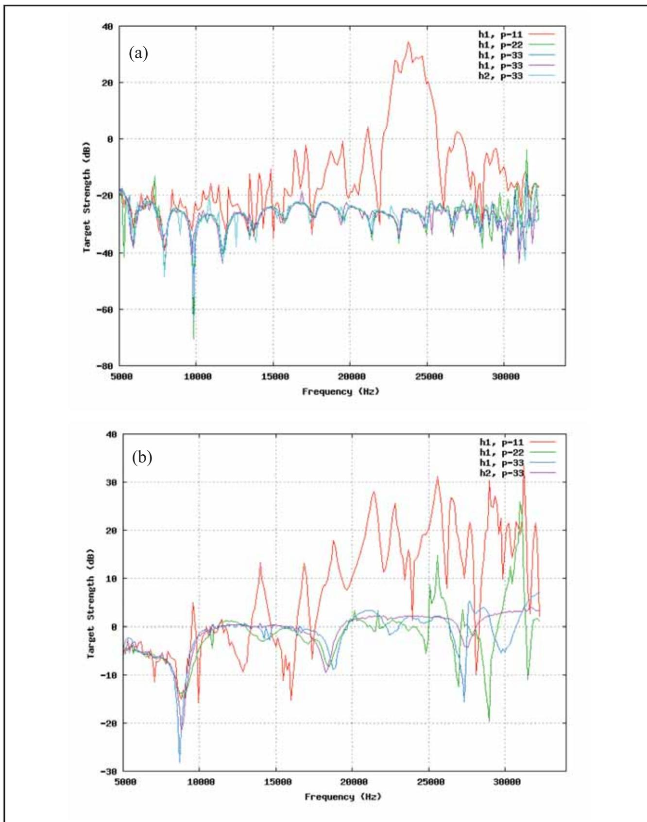
Figure 2. Effect of the  $hp$ -refinement in the scattering (monostatic response) from an E50 shell at (a)  $\theta = 0^\circ$  and (b)  $\theta = 90^\circ$ . Notice the convergence of the solution as higher order basis functions (indicated by the higher numbered  $p$ ) are used
