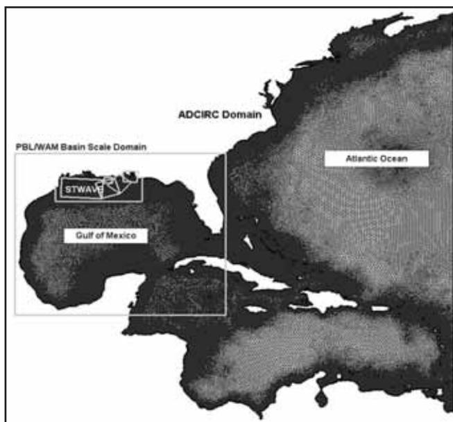
Figure 2. Model domains for system models: PBL, WAM, ADCIRC, and STWAVE
