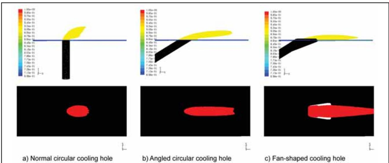
Figure 2. a-c Film-cooling jet structure for  $N_2$  injection
