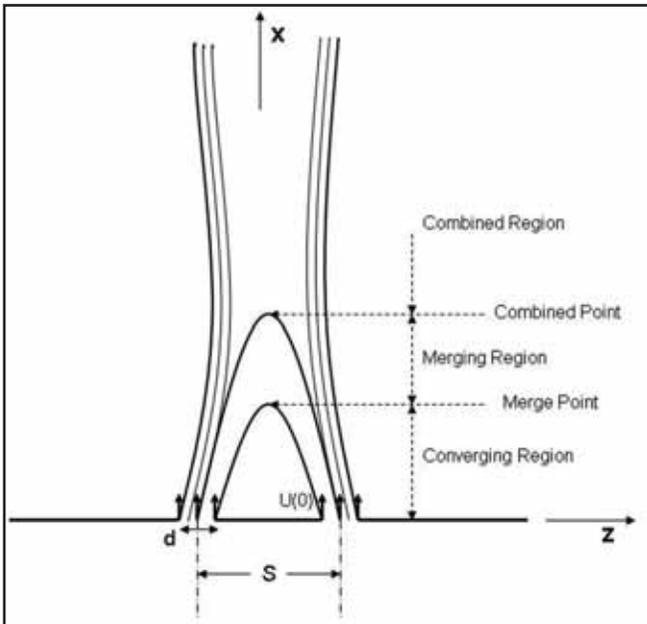
Figure 1. Parallel jet flow field regions and coordinate system
