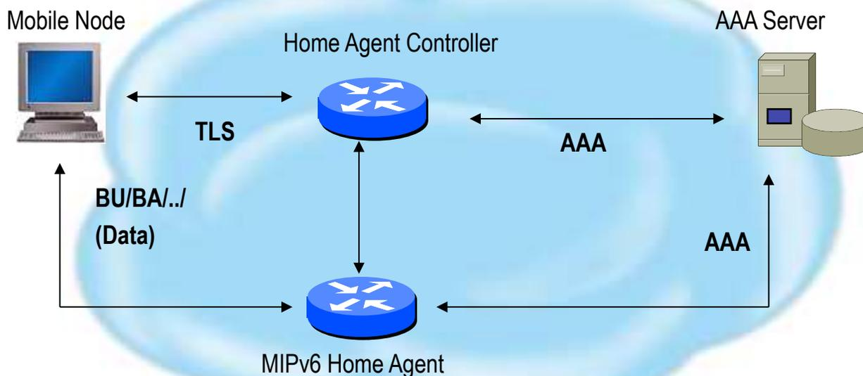
MN and HAC signaling message exchange protected by TLS
