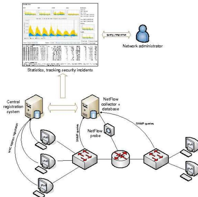
Figure 4: The Central Monitoring System for IPv4 and IPv6 at BUT
